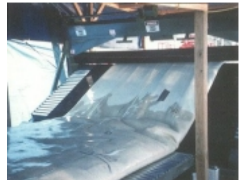
Resin is visible as the felt becomes saturated.
